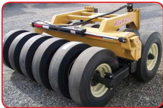
The unit shown is the WR90RL. This unit will Side-Shift 24" to the Right or Left. We also build a WR75R and a WR90R Hydra-Slide. These units Side-Shift 36" to the Right
