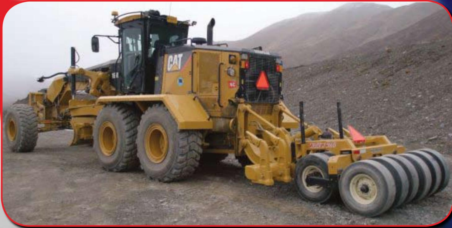
This is a WR90 **Walk 'n' Roll** Oscillator mounted on the rear of a 60,000 lb. 16M Caterpillar Motor Grader. The unit is working in Alaska.
